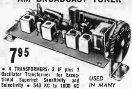
RADIOS! AN OUTSTANDING AM BROADCAST RADIO WHEN CONNECTED TO ANY TRANSISTOR AUDIO AMPLIFIER ON THESE PAGES OR ELSEWHERE!
