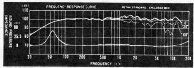
■ 20 TO 20,000 CPS (40 TO 16,000 CPS ± 3 DB) ■ HIGH EFFICIENCY ■ HIGH EXCURSION WOOFER WITH UNIQUE "CONICAL STIFFENER" ■ HANDLES HEAVY BASS PASSAGES WITHOUT "DOUBLING"
