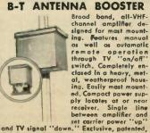
ing, Easily mast moni-ed. Compact pawer sup-ply locotes at or near receiver. Single line between amplifier and set carrier power "up" and TV signal "down." Exclusive, patented, 4 tube, push-pull circuit gives mare than 25db gain an all VHF channels. Matched 300 ahm inputs and autputs. Pawer Inputs for both 24 and 110 valts AC, Suilt-In filter net-
