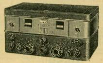
New communications receiver designed to provide the maximum in performance. Incorporates the latest, most desirable features. The 10-tube superhet circuit employs one tuned r.f. stage, two 455 kc. magnetite core i.f. stages with variable selectivity crystal filter, a.v.c., two a.f. stages with Degeneration in output New communica-
