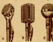
High quality, wide-range crystal mikes featuring: response from 30 to 10,000 c.p.s.; dual drive high capacity Graphoil Bimorph crystal ele-ments; barometric compensation; in-ternal screen protect-ed cartridges; output level 53 db. below 1 volt per bar; curvi-linear diaphragms; rich satin chrome fin-lsh; built-in cable con-nector and locking
