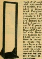
ed corners. Finished in ripple black. Designed for use with standard 19" long panels and are drilled for both Amateur and W. E. panel hole spacing. Baseis 16" deep, 20" wide. Holes are tapped for 10-32 screws. Base is braced to insure free-dom from wobble and to keep units in alignment. All heights shown below are overall dimensions.
