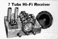
A fine 7 tube receiver that will give excellent results. The TRF circuit used is similar to that used in modern high fidelity receivers and will give excellent tone quality. Tubes used: 2-65K7, 1-6SJ7, 1-6SC7, 2-6G6G and 550 -5Y3.
