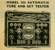
Modern tube tester and complete point-to-point set tester. Tests ALL tubes—new, old and future—under fullload, each element; "hot" leakage and short tests; double "floating filament" selector. Meter ranges: A.C. and D.C. volts: 7/140/700/1400; d.e. milliamperes: 1/7/140/-700/1400; ohms: 2000/20,000/2000,000; meg-ohms: 0/2/20 from internal power pack.
