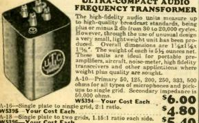
The high-fidelity audio units measure up to high-quality broadcast standards, being plus or minus 2 db from 30 to 20,000 cycles. However, through the use of unusual design a very small, lightweight unit has been produced. Overall dimensions are 1½x1½x1. The weight of each is 5½ ounces net. These units are ideal for portable pre-amplifiers, aircraft, noise-meter, high fidelity transceivers and other applications where weight plus quality are sought.
