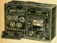
Combination free-point tester and volt-Combination free-point tester and voltohm-milliammeter. Complete in every detail for extensive voltage, current or resistance tests, either by direct contact with sockets or by the free-point plug-in method. Includes Triplett square-type, precision meter reading: 0-10-50-250-500-1000 volts, a.c., and d.c., at 1000 ohms per volt, (accuracy 2% d.c., 5% a.c.); 1-10-50-250 ma.: low ohms, 0-800; high ohms to 250,000 at 1.5 volts; battery is included.
