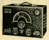
This improved version of a popular instrument introduced by Clough-Brengle to the service field now features air-tuned oscillator inductors, the type 6E5 cathode-ray tube for zero-beat indication, continuous calibration from 50 to 10,000 cycles and less than 1 db variation of voltage output across the entire frequency range. Wave form is guaranteed to contain less than 5 % distortion, which is less than can be observed by eye and well within tolerance.
