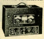
This instrument provides a calibrated output This instrument provides a calibrated output (in microvolts) for the accurate measurement of receiver sensitivity and gain. It employs a circuit providing uniform voltage output from 100 ke. to 20 me., readable directly in microvolts. The patented rotor-inductor assembly provides a frequency range of 100 kc. to 60 me. on fundamental output without the use of band changing switches or plussin industors. switches or plug-in inductors.
