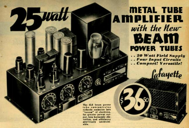
THE last word in modern public address amplifiers, the L Model 263-A uses all metal tubes (except for an 83 rectifier) in a circuit of such ultra-development that it was the first amplifier of its type ever made available to the public. Three 6C5's, two 617's and two beam power 616's comprise the tube complement, apart from the rectifier tube, an 83.
