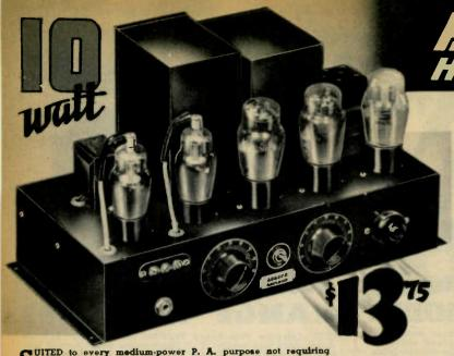
Suited to every medium-power P. A. purpose not requiring high amplification the Auburn 10 watt amplifier is particularly well adapted to amplified phonograph reproduction, to work with electric guitars and for general-purpose high quality amplification at low cost. Two input channels are provided, one for 200 ohm per button carbon microphone and one for high impedance input. Volume and tone controls are included.
