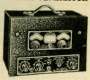
This instrument provides a calibrated output (in microvolts) for the accurate measurement of receiver sensitivity and gain. It employs a circuit providing uniform voltage output from 100 kc. to 20 mc., readable directly in microvolts. The patented rotor-inductor assembly provides a frequency repres of 100 kc to 60 mc. or fundes. a frequency range of 100 kc. to 60 mc. on funda-mental output without the use of band changing switches or plug-in inductors.
