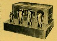
to the 50 tube with a resultant power output of 4.6 watts. The 2-81's, in a full wave rectifier circuit, provide ample plate current. Provision is made in the amplifier to supply the necessary field excitation for any 2500 ohm D.C. speaker.
