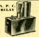
Suitable for any of the uses to which an extremely sensitive photocell relay may be put. Capacity 25 watts. non-inductive load. Adjustable for any desired light value. Operates normally open or closed. Requires standard photocell and -12A radio tube for operation. For either 110 volt A.C. or D.C. as specified in ordering.
