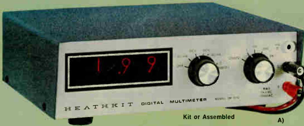
The all solid-state circuitry of the IM-1212 is contained on a single circuit board for easy assembly and access when servicing.
