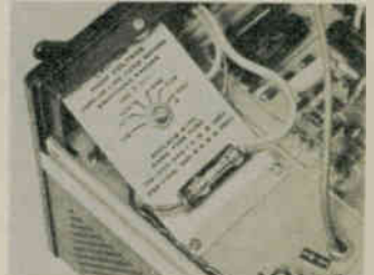
Adjustable line voltage switch matches the power supply of the IO-4510 to any voltage from 100 to 280 VAC.
