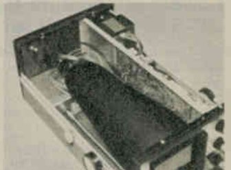
A complete mu-metal shield is used in the IO-4530 to eliminate display error caused by electromagnetic interference.
