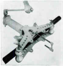
2PH or 2C Bender Up to 2" for 0° to 90° Bends
