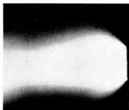
25% of beam is wasted in spill and glare.
