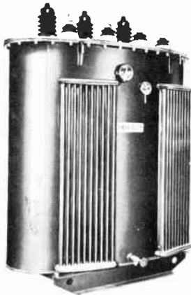
500 KVA oil immersed power transformer 3 phase 60 Hz 26400 delta - 4160Y/2400
