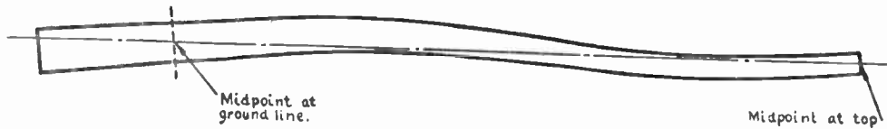
Diagram 2—Measurement of Sweep in 2 Planes (Double Sweep) or in 2 Directions in One Plane (Reverse Sweep)
