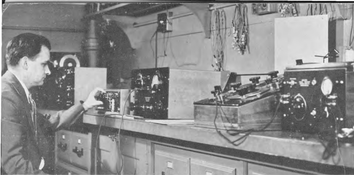
Above—Tests on an experimental model of Type 732-B Distortion and Noise Meter.
