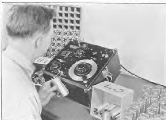
Production testing of electrolytic condensers with the capacitance test bridge.
