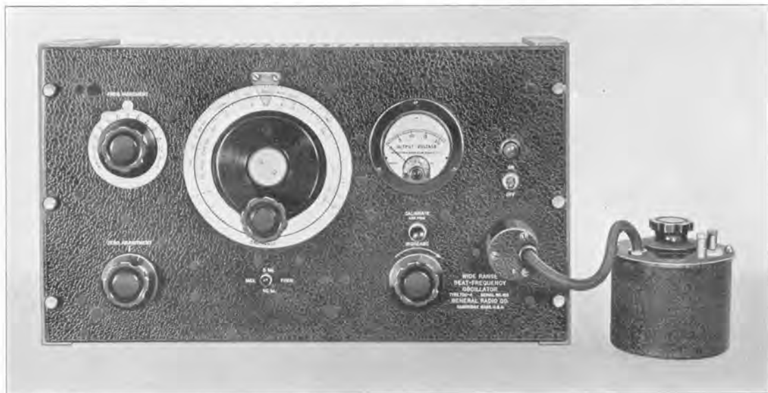
Panel view of TYPE 700-A Wide-Range Beat-Frequency Oscillator with TYPE 700-P1 Voltage Divider.
