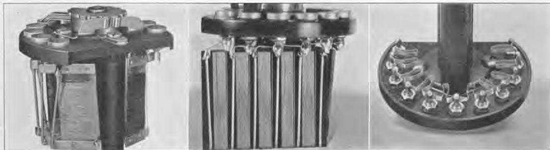
These photographs illustrate the methods of winding described above. (Left) Mica card method, (center) Ayrton-Perry method, and (right) Bifilar method.
