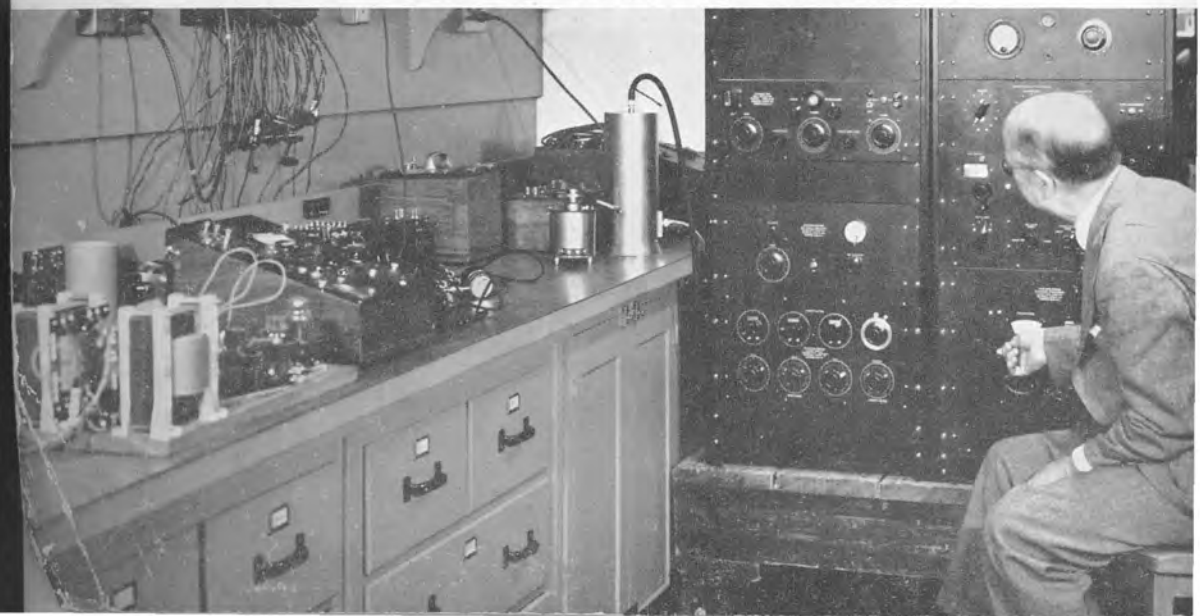
Above—Measuring frequencies with the General Radio Primary Standard of Frequency. Below—Engineering tests on a high-voltage, 60-cycle Schering Bridge.
