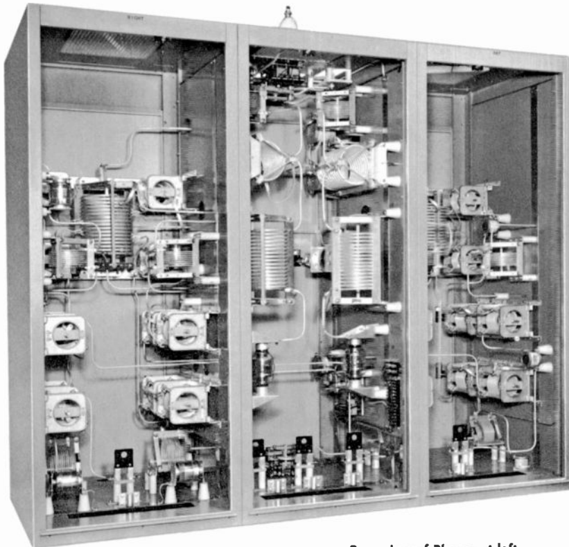
Rear view of Phasor at left, with panels removed. Note the clean mechanical layout.
