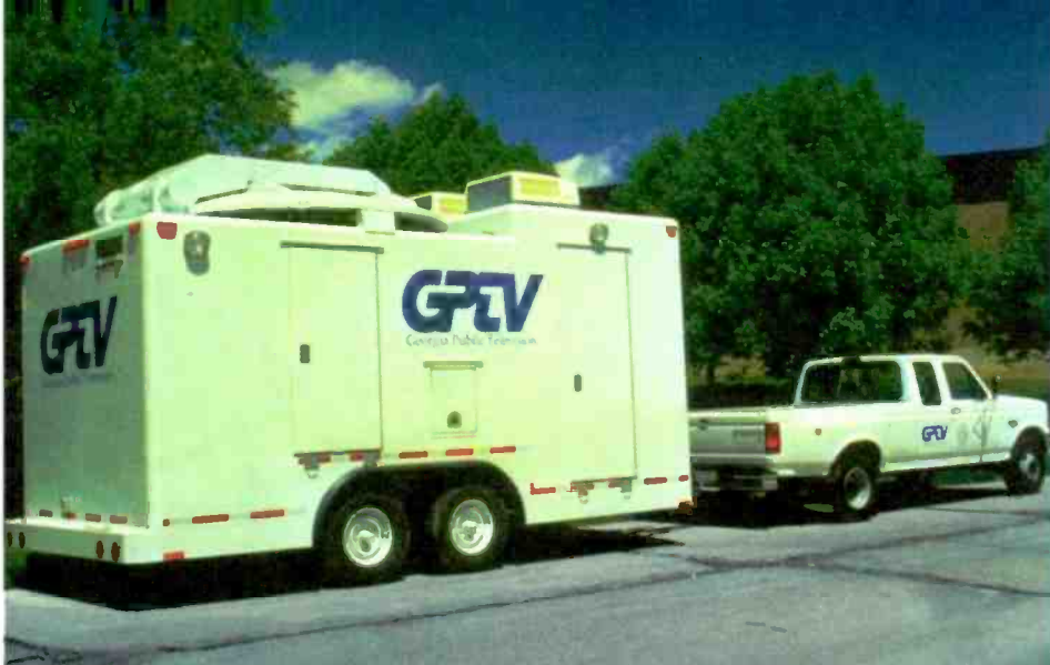
A unique trailerized satellite uplink system, the Harris S-20T is designed to be parked for days--or even weeks--on end. The tow vehicle provides ready local ground transportation for on-site crew.
