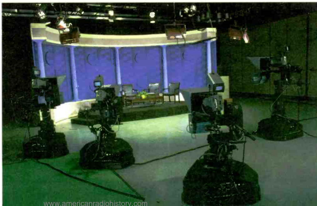
With robotic cameras, one person at a control console can perform live production functions that used to require three or four camera operators and a lighting technician.
