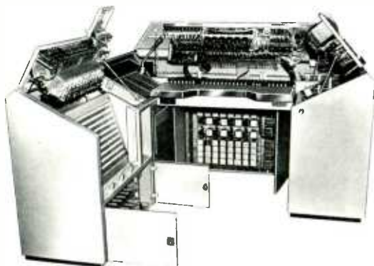
The above production console made for a leading television network houses 57 of the 6300 Series Solid Statesman transistorized units described herein.
