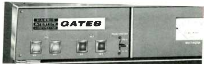
On-Off and multimeter switching functions are located on the top front panel of the FM-10G transmitter.
