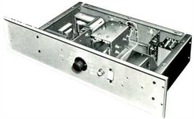
Built-in multimeter constantly monitors the operating conditions of the complete driver/modulator. A front panel switch permits instant switching from one oscillator to the other.
