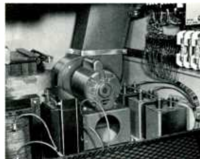
Blower provides 100% more air moving capacity than required. Incoming air is filtered through a washable air filter which can be changed while the transmitter is on-the-air.
