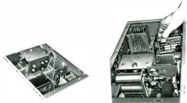
Solid state components are used in every stage except for the one tube final amplifier.
