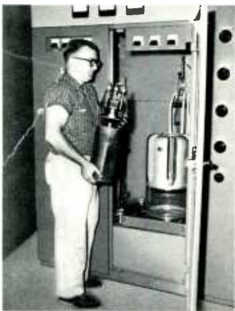
New F-8550 (PA and modulator) tube weighs 65 pounds and is a highly efficient, high-powered, long life, air-cooled tube. Standardization on this type tube for both the modulator and power amplifier permits interchangeability of tubes for longer useful life. This reduces the number of tubes required as spares and lowers the cost of operation.
