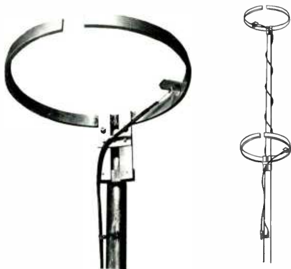
Left, FM11 single ring ammi-directional antenna with power gain of 0.8 db. Right, two bay FM-22 ammi-directional antenna with gain of 1.3 db. These are broad band, easy to install antennas.
