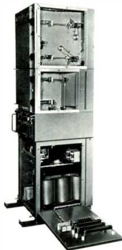
Mechanical tuning devices readily accessible from one side.
