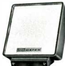
The M-6424 deluxe intercom sub-station is for studio use. Matches symmetry of console and particularly VU meter. Has 30° slant in cast aluminum housing finished in non-reflecting black.
