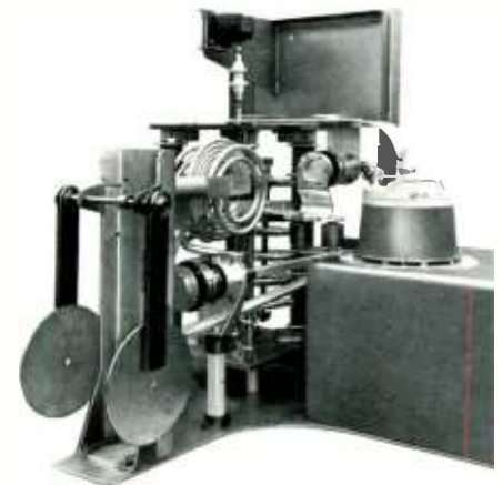
R.F. driver showing type 4CX15000 stage with grid circuits and cooling plenum.
