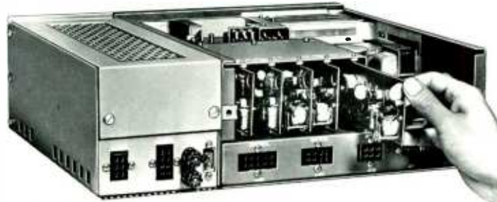
Rear view shows plug-in amplifiers which tailor system to meet individual requirements. Carritape II can be expanded at any time with additional plug-in amplifiers. (Fig. 1).
