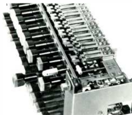
"Control Center" is built as heavy as the service demanded of it. Strong PBX type push keys with gold plated contacts automatically release if another is inserted. Handles are color coded and illuminated when circuit is in use. Control Center also provides voltage to operate mechanical devices. In "Control Center" two mixing channels do the work of 12.
