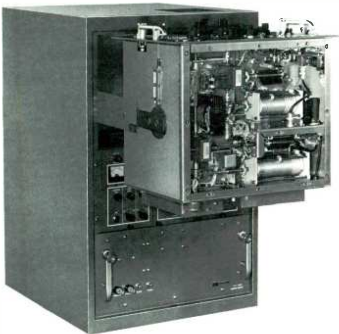
Note immediate accessibility to all service areas as a result of slide out tilt type construction.
