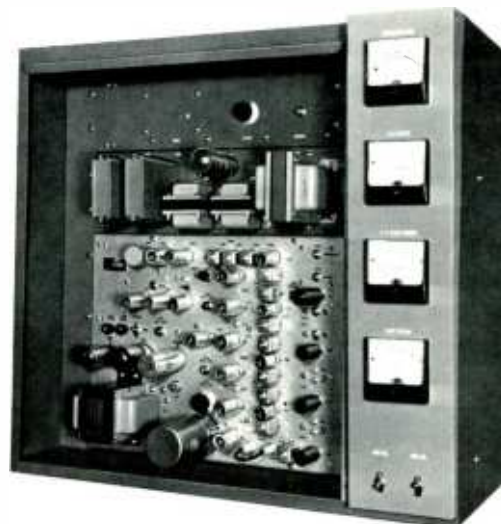
Front view (cover removed) of BFE-50C fifty watt FM transmitter.
