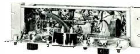
Right: Front panel drops down for easy servicing of all inner parts.
