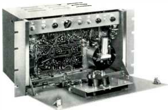
Front panel hinges down for maintenance and easy to reach operating adjustments. Note the circular temperature controlled oven containing all oscillator components and the precision vacuum type crystal. A rear slip-on dust cover protects tubes and terminations.
