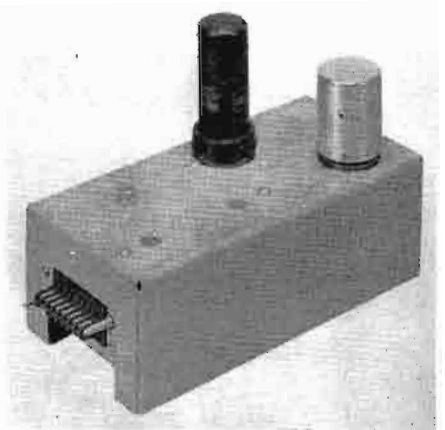
Individual view of one of the three plug-in oscillator units employed in the CMP-1 transmitter. Oscillators may be removed without disconnecting a wire and from the front of the transmitter.
