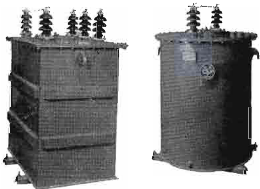
Modulation and reactor transformers are oil-filled and double impregnated, then mounted into gasket sealed steel tanks for indoor or outdoor service.
