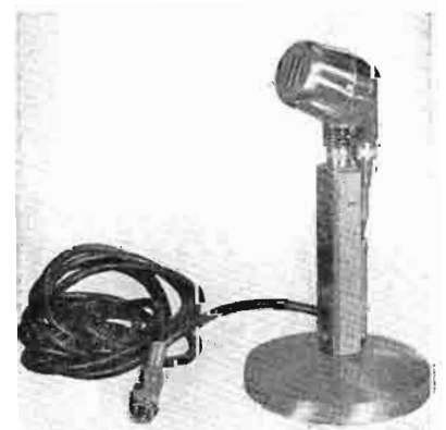
M-4576 dynamic microphone with push-to-talk desk stand, 7' cable and plug. Grip handle and transmitter turns on, release and it turns off. Output, -55 db. Hi-Z type.
