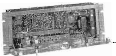
The front panel drops down to reach the muting relays. Two are standard but punch-outs are provided for three more if ever needed.
