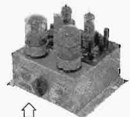
Dual vacuum mounted crystals are designed into a new oscillator with the emphasis on stability and dependability.
