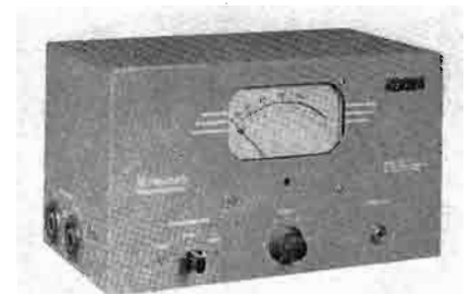
Left: Rear view of the Gates "Monomote". Cover quickly removes by loosening two snap locks. Printed wiring mounting board floats in rubber. Right: Front view illustrates the dual Cannon XL3-13 microphone receptacles. "Monomote" size is only 11" wide, 6½" high and 6½" deep, and weighs only 15 pounds complete.
