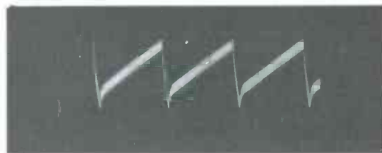
(g) V16, pins 1 and 6, 1.7 volts P-P, H rate
