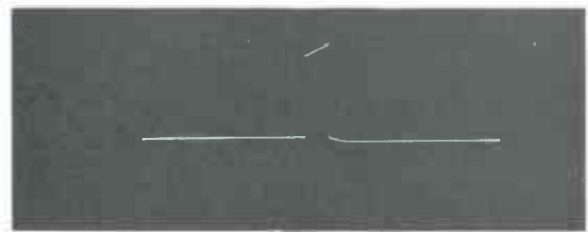
(f) V14, pin 6, 50 volts P-P, V rate
