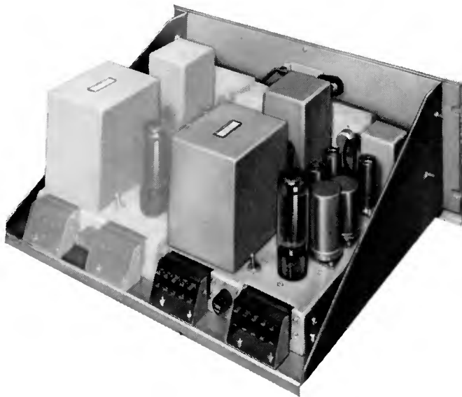
Rear view of FA-23-C Shelf, showing mounted BA-14-A Amplifiers.
