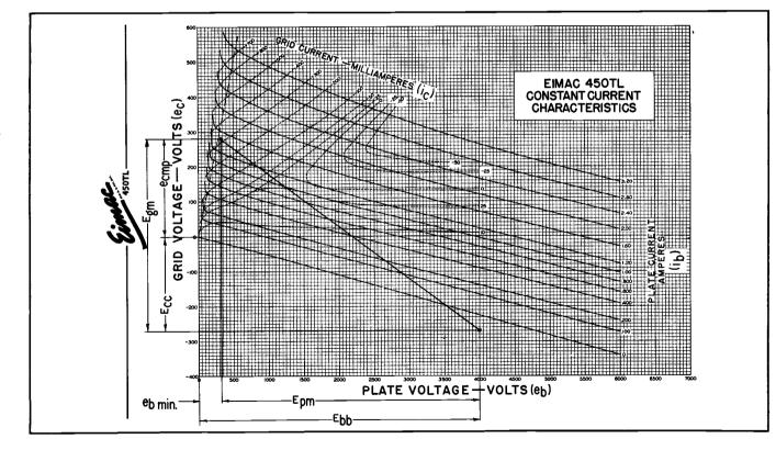
Figure 3. Method of determining e<sub>emp</sub> and i<sub>e</sub> on 450TL constant-current characteristics from values of e<sub>bmin</sub> and E<sub>pm</sub> found in steps 6 and 7 and value of i<sub>b</sub> found in step 10. The value of E<sub>ee</sub> and E<sub>gm</sub> from steps 13 and 14 and the operating line are also shown.
