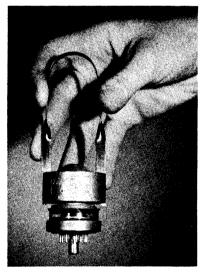
The Eimac 4X150 tube extractor may be used as pictured for inserting or extracting the 4X150A, 4X150D and 4X150G from normal or deep cavities. The prongs of the extractor are placed through the radiator of the tube and permit quick handling of tubes. The spring steel construction allows the tube to be gripped firmly without scoring the cavity walls. Only normal cavity wall clearance is required.
