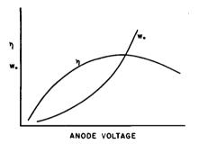
Fig. 5-Power output and efficiency versus anode voltage.
