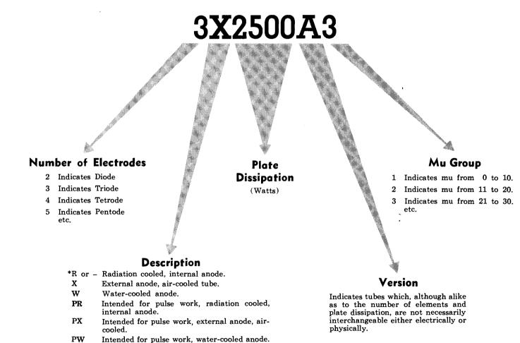
PW Intended for pulse work, water-cooled anode.
