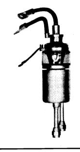
The Eimac 3W5000F3 is a water-cooled, medium-mu power triode intended for amplifier, oscillator or modulator service. It has a maximum plate dissipation rating of 5000 watts and is capable of high output at relatively low plate voltages. A single 3W5000F3 will deliver a radio frequency plate poweroutput of 7500 watts at a plate voltage of 4000 volts.
