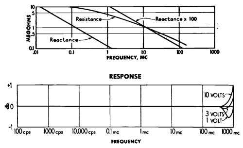
Input Impedance and Frequency Response of an Eimac 2-01C operating in a Hewlett-Packard Model 410B Vacuum Tube Voltmeter. Reproduced from Hewlett-Packard Catalog No. 21-A, 1952.
