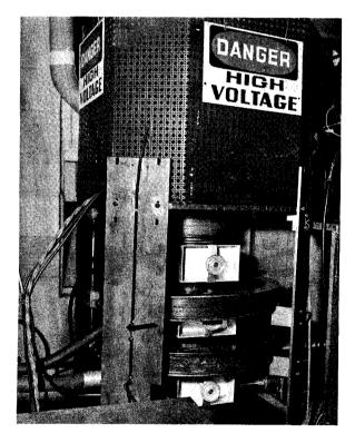
Fig. 8-The 5-kw klystron on test.
