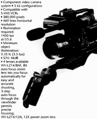
operates smoothly in both wide-angle and telephoto modes; WV-LZ15/12, 12X auto iris designed for studio applications; WV-LZ14/15 for a higher multiplication ratio of 15X • Optional 1.5X teleconverter can be used with WV-LZ14/8AF and WV-LA14/12A = Auto tracing white balance system = 2H enhancer with horizontal/vertical movement = Up to 1/2000 sec. electronic shutter speed = Interchangeable 35mm SLR and C-mount lenses with optional adaptor = Auto preset function
