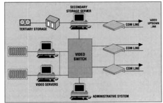
Figure 1. Video servers are used in conjunction with video switches, communication links, administrative systems and various methods of downloading content.
