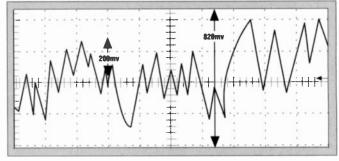
Figure 3. Time-domain display of an SDI signal that has passed through 1,000' of coax. Note lower amplitudes on shorter-duration pulses due to high-frequency attenuation by cable.
