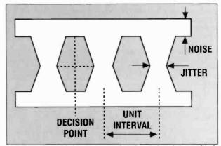
Figure 2. Once the serial datastream reaches the receiver, it is equalized. The amount of noise and jitter on the signal will determine the size and shape of the eye pattern, and if the receiver can properly retrieve the digital data.
