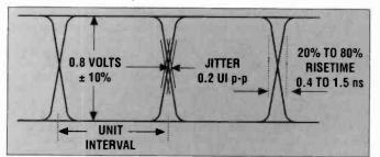
Figure 1. The waveform used for serial digital transmission has a peak-to-peak voltage of 0.8V  $\pm$ 10%. New specs call for jitter to be less than 0.2UI (unit intervals).
