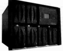
architecture • Support for RAID levels 0, 3 and 5 • Pushbutton graphical LCD display for on-the-fly configuration and monitoring Active backplane design • Hot-swappable and fully shock- and static-protected drive modules for data integrity
