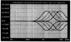
Figure 1. The mid-range curve is characterized as a haystack for boost and a *dip* for attenuation.
