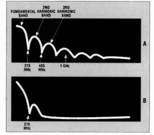
Figure 2. The spectrum shown in (A) represents a healthy SMPTE 259M (component) signal, while (B) shows the same signal after passing through 1,000' of coax.
