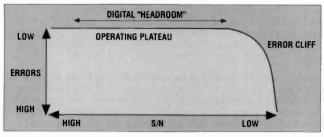
Figure 1. All digital systems experience the "cliff effect" in which performance remains optimal until S/N degrades beyond a certain limit.
