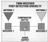
Figure 1. Non-active antenna diversity uses widely spaced antennas that are passively mixed by the receiver.
