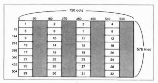
(Figure 5: Recorded Pattern of Index Picture [PAL])
