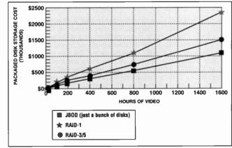
Figure 3. Media cost differences between various disk storage systems.
