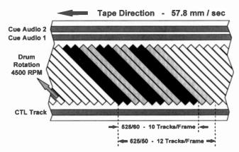
The system uses a two-track, parallel recording system with a pair of heads on each side of the drum, aligned exactly opposite each other (180°).
