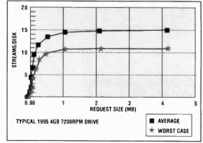
Figure 2. Average and worst-case performance of a 7,200rpm drive when supporting multiple 3Mbps video streams.
