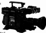
eliminates the need to use menu setup when using RU-Z1 or RU-Z2 control units - Character display on camera head video output allows the menu to be displayed on a large monitor for easy viewing and operation
