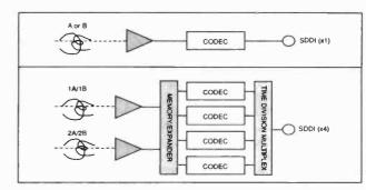
(Figure 7: Signal process for high-speed data transfer)
