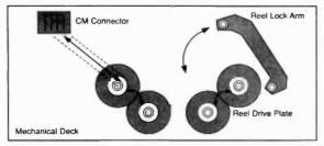
(Figure 6: Dual Cassette Mechanism)
