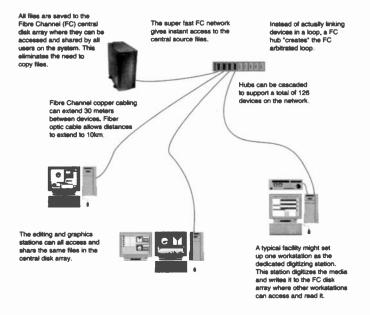
Figure 2. A Fibre Channel Configuration in a Typical Post-Production setup
