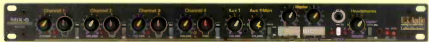
MIX-6 • 6 stereo inputs. Inputs 1-4 are XLR/TRS mic/line, 5 is aux RCA, 6 is aux TRS.
