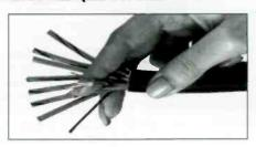
Star Quad gets its name from the four-conductor style construction that minimizes the "loop area" between twists of the conductors, reducing susceptibility to noise. It's designed for use with mics but is also excellent for all line-level signals. Buy it by the foot or in two reel sizes.
