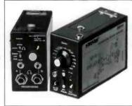
This compact, battery operated mic-to-line amplifier provides gain of up to 84dB, adjustable in 6dB steps. The unit has both a balanced XLR mic level input and a 1/8" TS mini input for a high level, high impedance source. The output is transformer balanced and appears on both an XLR connector and a set of spring contact binding posts. A very smooth switchable peak limiter and belt clip are included in this rugged, dependable unit. Powered by a single 9V battery.
