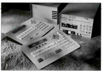
The RC-220 Remote, designed for production work, duplicates the machine's front panel and includes 16 presets for instant playback and a keypad for rapid cut selection. Controls up to four machines.
