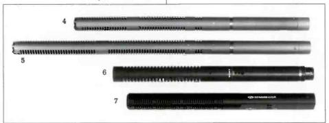
pole. Long shotguns are best used for sound sources at a distance. Short shotguns are recommended when sound sources may be closer and may have a tendency for moving "off-mic."
