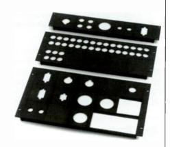
Middle Atlantic has developed a unique way to have custom panels without the cost and time of custom fabrication. Frame kits, which have rack ears and mounting bars, come in sizes from two to ten spaces. Punched modules, which are two spaces high and fit five across a rack, are provided punched for your choice of connectors. Combinations are unlimited. A fully loaded two space frame is less than \$60. Call or fax today for details.
