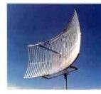
beamwidth of 19° (horizontal) and 10° (vertical). It weighs only 30 lbs. (including feed and mount), and utilizes universal clamps for quick installation on pipe diameters from 1.9" to 3.5".
