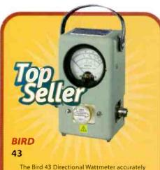
measures forward or reflected power in coaxial transmission lines under any load condition. Each model 43 consists of a line section, "QC" (Quick Change) connectors and an indication meter housed in a rugged, corrosion-resistant aluminum case. Plug-in elements, purchased separately, determine the power rating and the frequency range. Elements can be purchased at any time and replaced in the field. Call for pricing on the elements for your application.
