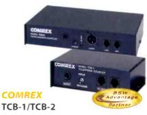
TCB-1 broadcast coupler sends and receives program material via the switched telephone network. This unit requires no external power and connections are via standard modular plugs. The TCB-1 contains an FCCregistered coupler which provides isolation from hazardous voltages and currents and includes an active circuit to hold the telephone line. Includes 1/4" jack for line level input.
