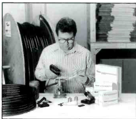
A BSW technician prepares a custom cable from in-stock components at our Tacoma facilities.
