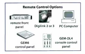
DL4 can be controlled from the built-in control panel with LCD display and two other control ports at the same time. Control the DL4 via the optional 99 button Gemini control panel, PC via modem or locally; a Digilink workstation; optional GEM-DL4 console module (fits 12,000 and 22,000 series consoles); optional remote LCD control panel that duplicated the DL4 front panel.
