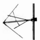
The JHCP antenna is a circularly polarized FM antenna for the broadcaster who wants extremely high-input power capability, coupled with the patented design that has become an industry standard. This design is sophisticated in concept yet simple in execution. Each bay consists of a radiating element with its associated 6 1/8" (15.56 cm) interbay feed line. The element and line are supported by a heavy brass casting which is attached to the support structure by its mounting bracket.
