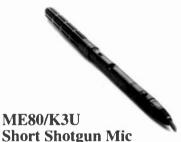
Combination of supercardioid at low frequencies, and shotgun above 2,000 Hz. Excellent on-camera or hand-held interview mic for ENG/ EFP. Use with K3U power module. Frequency range 50-15,000 Hz.
