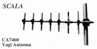
The CA7460 is a seven-element yagi designed for high performance and long-term reliability even under severe environmental conditions. Its broadband design makes it particularly suitable for systems requiring frequency agility within a specified band. Two standard models cover the 406-420 MHz and 450-470 MHz bands. Custom models are available for other portions of the 200-500 MHz spectrum. Impedance is 50 ohms, gain is 10 dB (over dipole), and input power rating is 100 watts.
