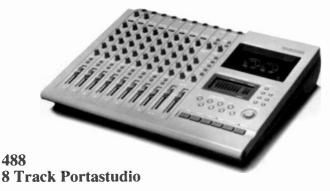
The 488 Portastudio is a compact 8-track cassette/mixer studio that is both easy to use and affordable. Features: 2 mono mic/line inputs, 6 mono and 2 stereo line input, 4 independent group outputs, 2 effect sends, 2-band EQ on channels 1-8, auto locate to 2 memory points, 8-track and stereo metering, dbx noise reduction.
