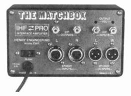
The Matchbox is the ideal, inexpensive way to correctly interconnect "HI FI" or simi-pro equipment with professional studio gear. The Matchbox is a bidirectional unit with four independent amplifiers providing full stereo input and output interface. Features adjustable output levels.
