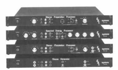
The FM-4G System is a careful blend of superb sounding stereo multiband AGC's, low distortion pre-emphasis limiters, and overshootless low pass clipping filters which make outstanding quality and loudness improvements easy to obtain.
