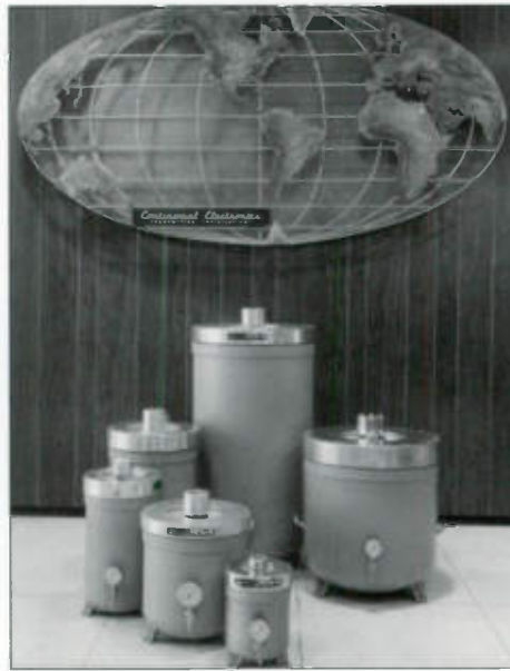
Top Left: Variometer used for tuning of 2 megawatt VLF/LF antenna system.
