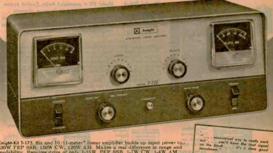
Knight-Kit 7-175. Six and 10/11-meter\* linear amplifier builds up input power too 330W PEP SSB, 150W CW, 120W AM. Makes a real difference in range and readability. Requires drive of only 1-15W PEP SSB, 1-7W CW, 1-4W AM.
