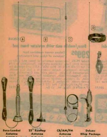
A-2581 Base-loaded Antenna, Easy-mounting antenna with stainless-steel shock-spring for low garaging. Triple-chromed dress cup and no-hole "Quick-Grip" trunk mount. Easily removed —leaves no scars. Tapered stainless-steel whip with fine-tuning adjustment for perfect match to 50-ohm output. Height, 45". Solderless 16-ft.
