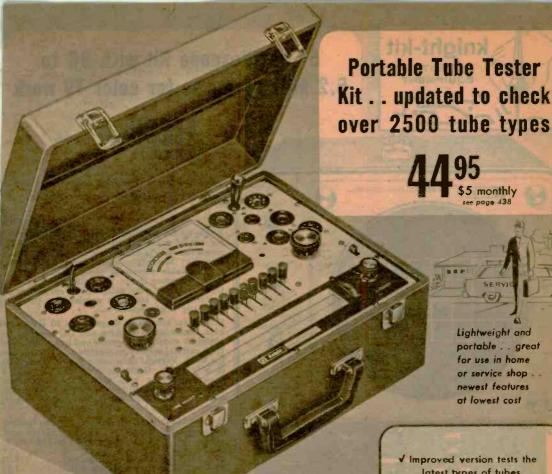
Knight-Kit KG-600C. Improved version of our popular KG-600B emission-type tube tester kit updated to meet today's complex radio and TV servicing needs. Accurately checks over 2500 tube types, plus many CRT's (with optional harness below), and pilot lights to 117 V. Features illuminated roll-chart for fast, easy sctup; easy-action universal-type selector switches; easy-to-read 3-color 4½" meter; sixteen different switch-selected filament voltages from 0.63 to 117 volts.
