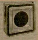
Musicaster 1A. All-weather speaker for outdoor PA or extension uses. Has 12" wide-range driver for good bass response; Radax dual-cone driver assembly for crisp highs. Compression molded housing. Universal "U" bracket for easy mounting. 80-10,000 Hz. Dispersion: 120°. Power than the property of the pr
