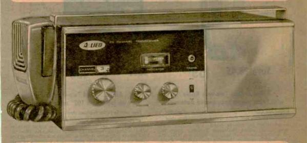
Operates on either 12 VDC for mobile or 117 VAC base from built-in power supplies electronically regulated to provide maximum stability over a wide variation in input voltages
