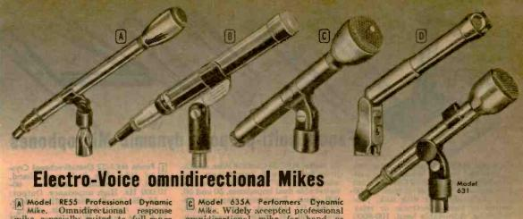
Mike. Omnidirectional response mike especially suited to full-range music recording and other exacting professional applications. For hand and stand use. Pop-proof; built-in blast filter. Response is extremely stable; mike can be calibrated for use as secondary lab standard. 40-20,000 Hz. 150 ohms, Output: -55 dB. 18' three-conductor cable. Satin nickel finish. 10\(^1\)2x1\(^1\)\dagger^2, \(^2\)4' shank. 12 A 7250. Wt., 14 lbs. . . . . 126.00
