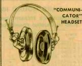
COM.S. Extremely sensitive head-COM-S. Extremely sensitive head-set for all communications use. Lightweight, fully adjustable head-band; vinyl-covered foam filled ear cushions. Dynamic elements for crisp, clear reproduction. Response: 100-10,000 Hz. Impedance: 4-16 ohms. Supplied with 7' two-conductor cable with ¼" phone plug. Shpg. wt., 11b.
