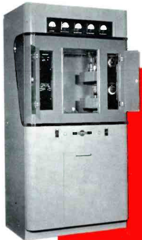
Collins 300J 250 Watt Broadcast Transmitter
