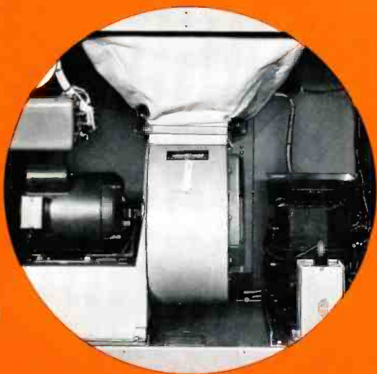
POWER AMPLIFIER CABINET BLOWER
