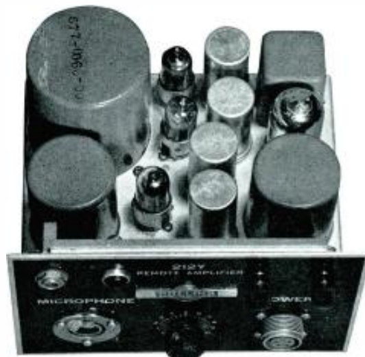
The cover can be removed by loosening a single fastener.
