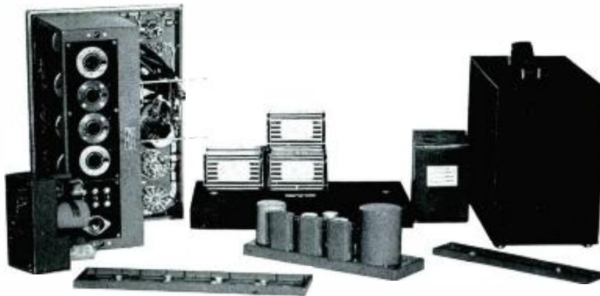
The 12Z can be disassembled easily and completely, requiring only small hand tools. Unit construction has been used advantageously for simplicity of maintenance.
