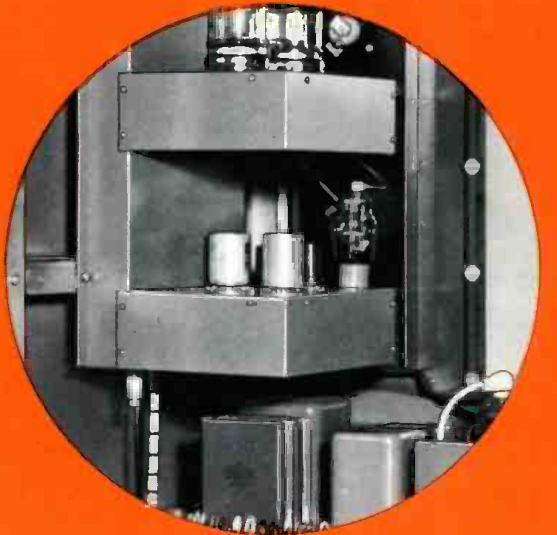
DRIVER CABINET RF CHASSIS
