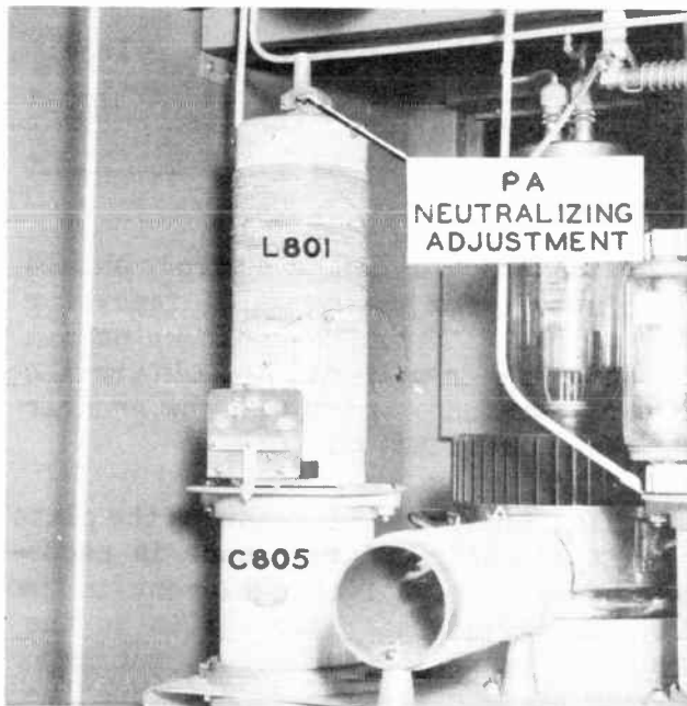
Figure 3-3 Neutralizing Coil Adjustment
