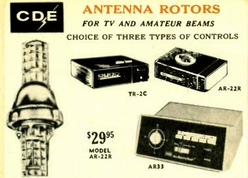
**HEAVY DUTY ROTOR UNIT.** First choice of thousands! Rotates full 375 degrees at approximately 1 RPM with positive, automatic stop in either direction. Instant reversing, Built-in 61/2" diameter ball thrust bearing will handle heavy antenna ... no additional bearing support needed. Clamps take 7/8" to 2" dia. Mounts also on flat surface when lower mast support is removed. Mechanism has oilite and ball bearings, lifetime lubrication. Shop, wt. 15 lbs.
