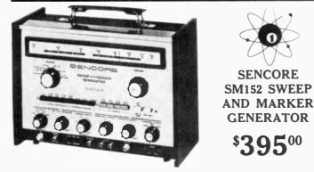
All solid state. The SM152 can completely sweep align the UHF tuner, the complete VHF tuner, the IF, and the chroma bandpass. Each stage can be aligned individually, or the entire signal system can be aligned for a correct overall response. Sound, video, color, and all trap markers "pop" singly or simultaneously on the response waveform. Only 3 hook-up cables are required; one for RF signal in, one for detected signal out, and one for the
