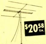
Uses 4 elements—2 directors, a double tolded dipole and a reflector with length and specing of elements set by foctory for optimum gain and performance on one channel, though considerable gain may be expected on adjacent channels.
