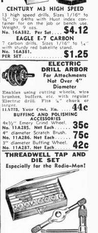
A tool set of the highest industrial quality—designed to fill a long-felt need in radio and hobby work. Con-tains just the sizes needed. Each die is provided with a pressed steel guide is provided with a presed steel guide that assures a perfectly straight thread. Set contains one tap and one die of each following sizes: 2-56, 4-36, 4-40, 6-32, 8-32, 10-32, 12-24, 1/4-20; eight threading guides; a tap wrench and a die stock—all in ma-chinists' type wood box. **16A541. Your Cost, Net**
