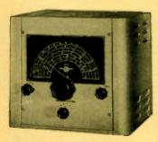
For added sensitivity, image rejection and gain when used with any communications receiver. Range 550 KC to 33MC. Built-in power supply. Tubes are 2—6K7 and 1—80. Cabinet matches current RME receivers in every detail. Operates on 115 V. 60 cycle AC.
