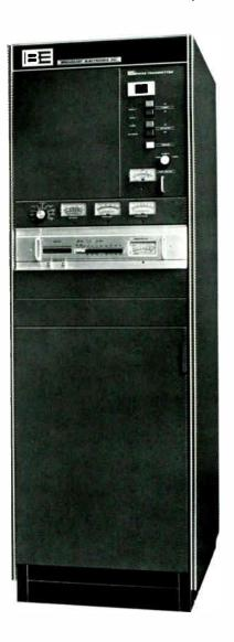
BROADBAND, SOLID-STATE IPA — A single broadband module using one (1) Type CD-4262 palanced RF power transistor serves as the IPA in the FM-3.5 transmitter. This driver module is conservatively operated at about 50% of its maximum rating, so there is plenty of reserve power in the IPA stage.
