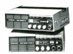
UHER 4000 Report IC (Mono) — This is the world-famous battery-operated, portable hi-fi open-reel tape recorder (DIN 45 500), of proven excellence even under extremely adverse operating conditions. Has rugged, reliable construction. Frequency response 35-20,000 Hz. Wow and flutter 0.2%. The machine is equipped with longlife Recovac tape head (triple life). 2-track mono operation. Compact housing of diecast aluminum. Metal knob and
