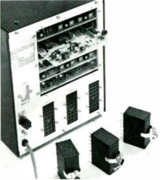
Electronics for the decks are on individual plug-in pc cards. Also shown above are the mating connectors which are supplied with the machine. The record connector is in place (above the fuse holder) behind a protective shield.
