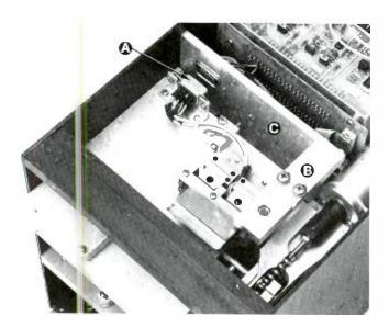
The 5300.  $\mbox{$^{\uparrow}$}$  front panel is hinged, the decks pull out, and all electrical connections to the deck are made through a single plug in connector (A).
