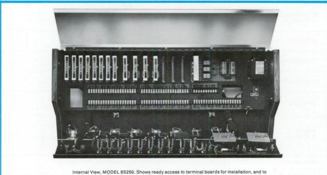
Internal View, MODEL 8S250. Shows ready access to terminal boards for installation, and t attenuators, switches, modules and all components for service and maintenance.
