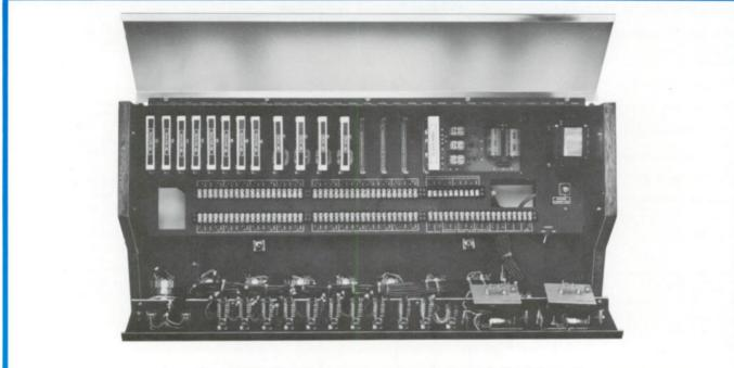
Internal View, MODEL 8S250. Shows ready access to terminal boards for installation, and to attenuators, switches, modules and all components for service and maintenance.
