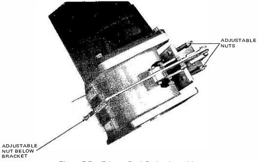
Figure 5-7. Takeup Reel Brake Assembly
