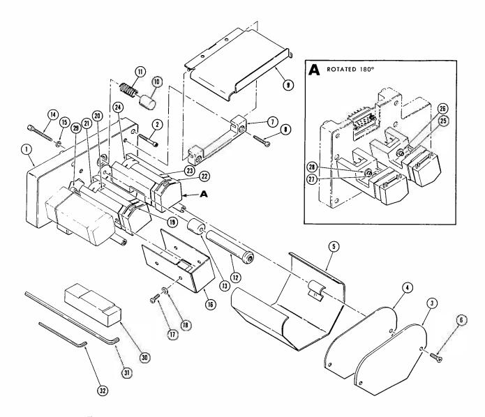
Figure 5-12 Audio and Cue Head Assembly Exploded View
