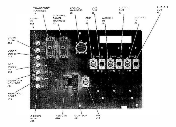
Figure 2-3. Signal and Power Connections
