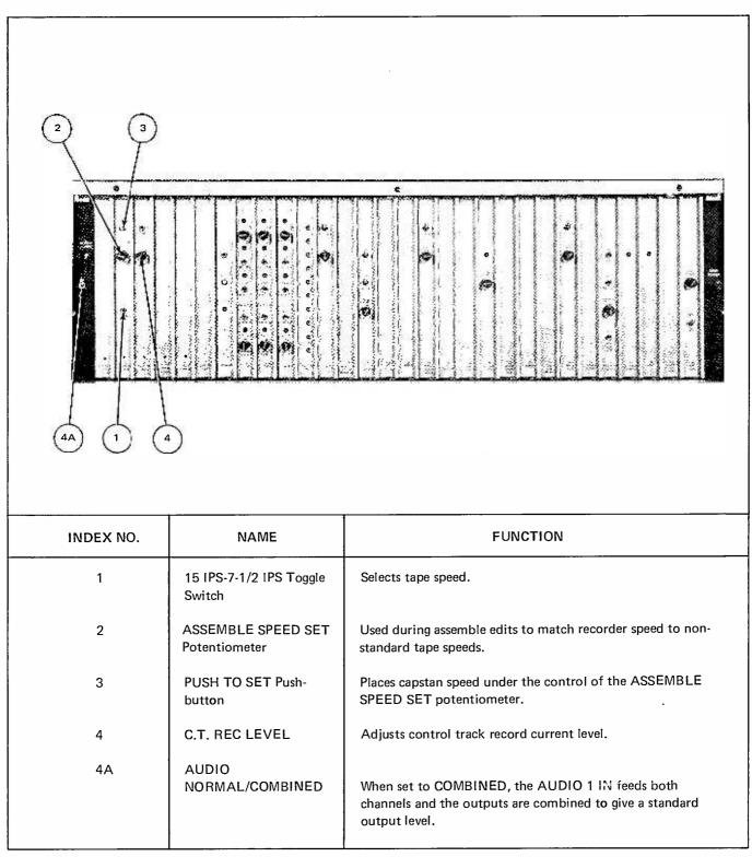
Table 3-6. Card Rack Assembly Switches and Controls
