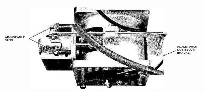
Figure 5-8. Supply Reel Brake Assembly
