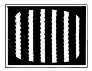
Figure 5-4. Picture Scalloping of Vertical Bar Test Signal
