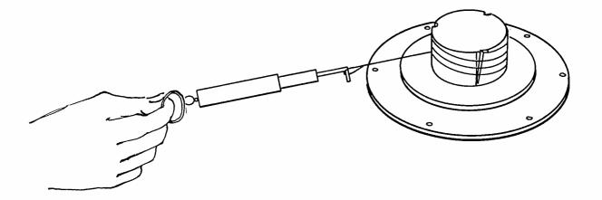
Figure 5-5. Preparing for Reel Tension Adjustment
