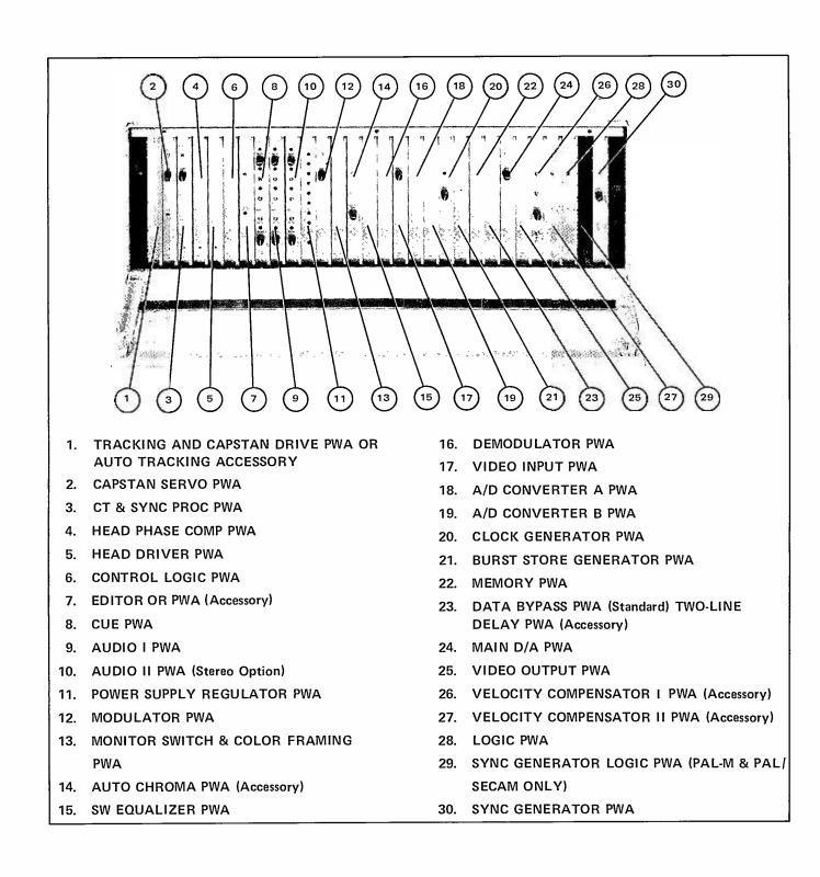
Figure 1-6. Electronics Assembly
