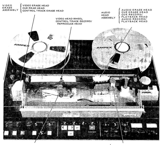
VACUUM GUIDE ASSEMBLY MONITOR CONTROL MONITOR HEAD AUDIO MONITOR
