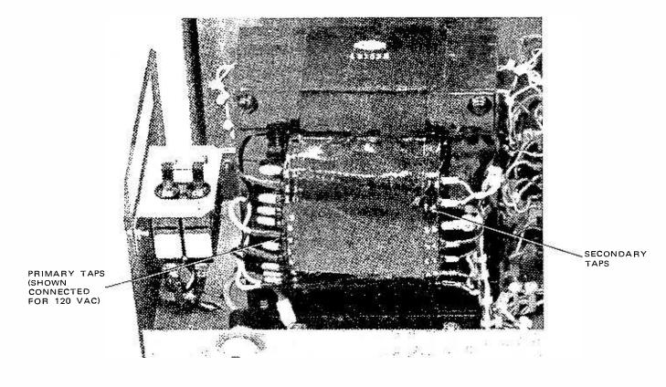
Figure 2-4. Power Transformer Tap Connections
