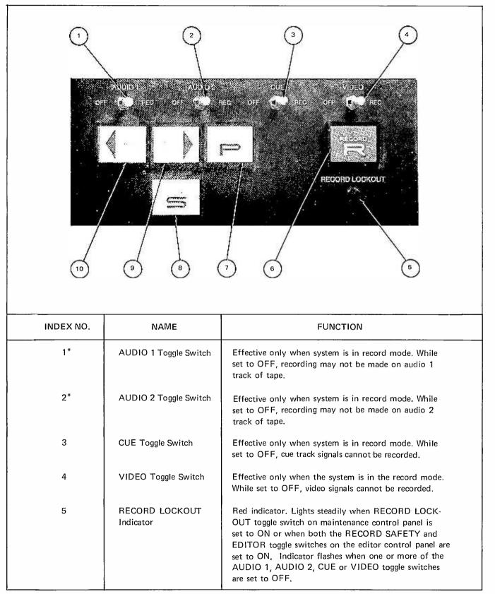
Table 3-1. Control Panel (Middle Section) Operating Controls and Indicators
