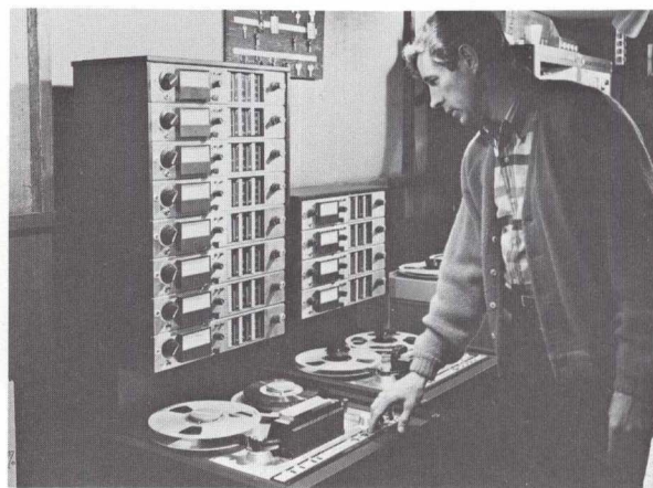
Using an Ampex AG-440 eight channel multichannel recorder, Charlie Tallent is able to make a recording in stages, perfecting each stage as he goes, and still come up with a first generation tape. Three other AG-440's, in four, two and one channel versions are also used at The Barn.
