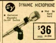
Ideal for public address or recording application. Response: 60-15,000 cps. Output: —55 db. Has four-stage blast filter to reduce "Pop" 16' cable. Size: 6\%2 x 1 25/64". High impedance. Shipping weight 3 lbs.
