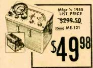
The Model 117B has sixty times the sensitivity of a Geiger counter. The detecting element is a 1" diameter x 1/2" thick Thallium activated Sodium lodide crystal hermetically sealed and optically coupled to an RCA 6199 photomultiplier tube. The tube and crystal assembly is enclosed within the instrument case and is magnetically shielded. Operating ranges of the Model 117B are .025, .05, .25, .5, 2.5 and 5 milliroentgens per hour. Shipping weight 11 lbs.
