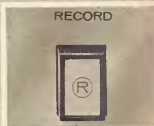
Record Interlock Button Prevents Accidental Erasure of Your Tapes
