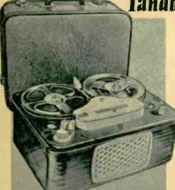
Deluxe, 3-speed, portable recorder for play-ing recorded 2 and 4-track stereo and monophonic tapes—and for making 2 and 4-track monophonic recordings. Operates at 1½, 3¼ and 7½ ips. Responses 30-17,000 cps at 7½ ips. Precision-built tape mechanism features low tape tension, minimum wow and flutter, and extremely quiet operation for superior performance.
