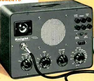
Perfect for extremely fast, convenient signal tracing by aural and visual methods—traces IF, RF, video and audio circuits. Exceptionally high amplification. Gain of 91,000—highest by far, in its price class.
