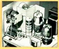
Deluxe components used throughout, oversize power transformer . . . ceramic coil forms . . . 807 transmitting tube . . . ceramic-Insulated, true transmitter-type variable capacitor in final amplifier.
