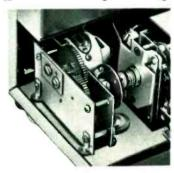
the internal switch to the proper range, and a light immediately flashes on the front panel to indicate the scale range in use. There's no need to set any manual range switch-valuable time is saved by the fast-acting motor movement. Exceptionally dependable nylon gears are employed to provide extremely smooth, quiet operation. Range switch can race through all 11. ranges in less than 21/2 seconds, automatically and efficiently. Unit can be locked into any range by a flip of a switch!
