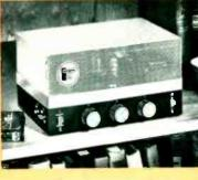
Built-In Equalized Preamp for Magnetic Cartridges, plus Separate Bass and Treble Controls
