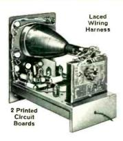
Two up-to-the-minute printed circuit boards for quick, easy, error-free assembly; laced wiring harness even further reduces assembly time.
