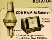
Heavy-duty rotator system for control of large antennas in high winds. Features rugged brake and motor with stainless steel gears and 98 ball bearings. Has end-of-rotation power cut-off. Vertical load rating over 1000 lbs.—heavy plates distribute stresses. Indicator can be read with-out starting motor. Meter calibrated with com-
