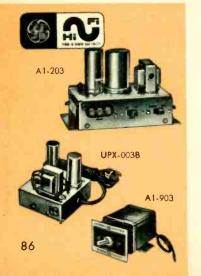
A1-203 "TRANSISTUBE" PREAMP. Allows using mike or any magnetic cartridge with ampli-fiers not having necessary inputs. Extremely fiers not having necessary inputs. Extremely low hum, noise and microphonic levels Uses 12AX7 and NPN transistor. RIAA cartridge equalization. Includes gain control. Has 3 input impedances, 2 sensitivity positions. 10 my sensitivity for 1 v. output. 3½x3½x6°. With 2-ft. cable, For 110-120 v., 50-60 cycle AC. Slpgs. wt., 3½ lbs. 81 \$ 857. \$2.00 Down. NET. 21.51
