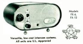
ALL-MASTER SYSTEM, Consists of up to 6 FX 6 (or 12 FX-12) Masters —np to 3 (or 6) private conversations can be carried on simultaneously, Individual slide switches on FX-6 permit conterence calls. A Master can be called even if its power is off; stations can be placed up to 2,000 feet apart. Use 7 cond. cable from 1st FX 6 to 2nd, 2nd to 3rd, etc.; use 18 cond. cable between FX 12's.
