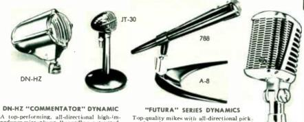
pedance microphone. Ruggedly constructed, the "Commentator" features a handy, tilt-ing-head swivel mount. An ideal unit for all general purpose semi or non-directional ap-plications. Frequency response, 50,7000 cps. Output level, —55 db. Handsomely finished Output level, -55 db. Handsomery ninsneu in opalescent gray baked enamel with gleaming chrome grille and trim. %6".27 threaded mounting, 10-ft, cable, Wt., 234 lbs. 99 \$ 304. List, \$39.70. NET .... 23,34
