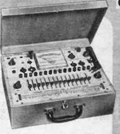
Deluxe model combines mutual conductance (Gm) and plate conductance (Gp) tests with peak emission test—gives single reading of tube quality. Numerical and quality zone scale readings. Tests all standard tube types, plus special purpose, VR's, cold cathode regulators, electron-ray indicators. Gain, leakage test for transistors. 4½" meter; multicircuit level switch. Roll-chart for easy setups. Latching case- $4\frac{1}{2}$ x15x12'. For 115 VAC.
