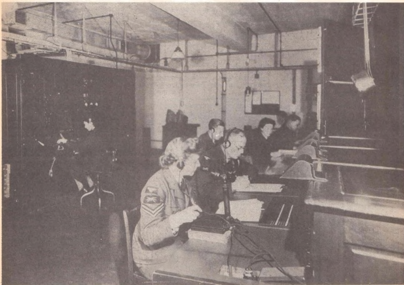
Fig. 5. An operational CH radio location receiving room and equipment. The WAAF operator at the receiver unit (left) determines direction and distance of enemy aircraft. Relevant information is then passed to command control. Copyright. Imperial War Museum.
