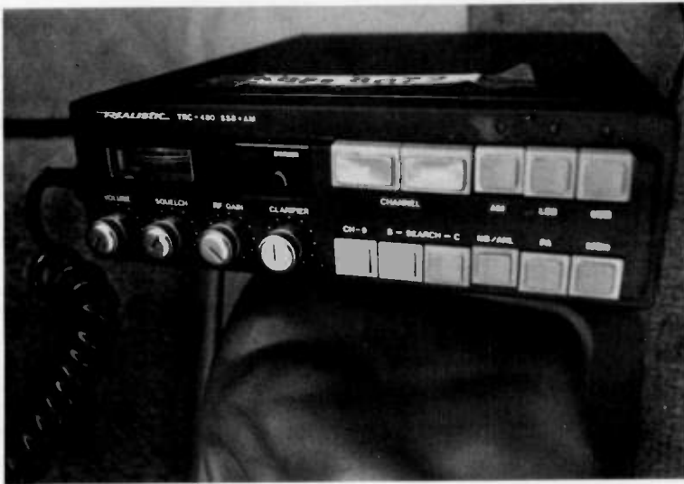
An alternative might be mounting your rig by the stick shift, but remember that you might run into problems with hitting your rig when you shift.
