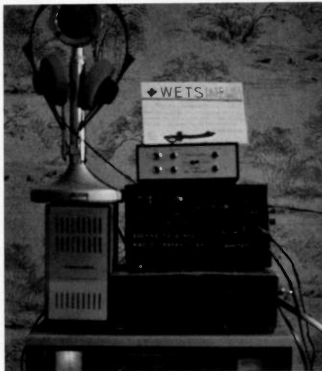
In the well equipped studio of WETS Radio are this DX-160 receiver and speaker, T250-30A frequency counter, D-104 microphone, Realistic stereo preamplifier, Sennheiser stereo headphones, and homebrew transmitter. A WETS QSL card is on top of it all.
