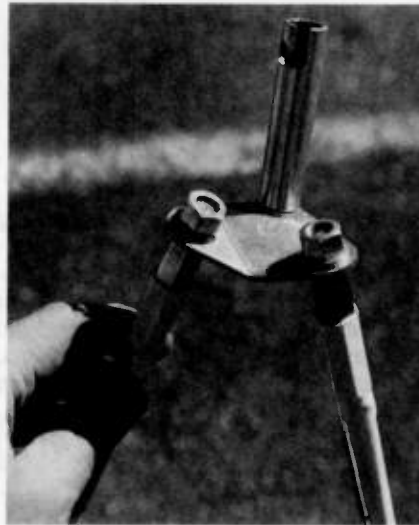
3. The V-MOUNT is attached to a quick-disconnect mount for easy removal.
