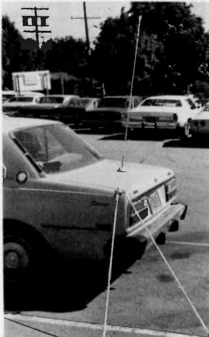
6. If you have a third (single) stick antenna, you may change from it to the V-Beam whenever you wish—use the V-Beam for the highway and the normal stick for driving around town.
