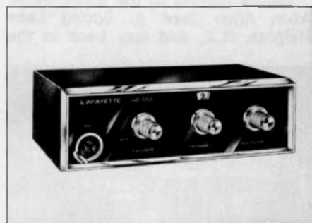
The HB-555 was Lafayette's approach to a miniaturized rig (mid-1960's) when most sets were big and bulky. It wasn't much of a performer but it was one of the first really compact rigs ever mass marketed.
