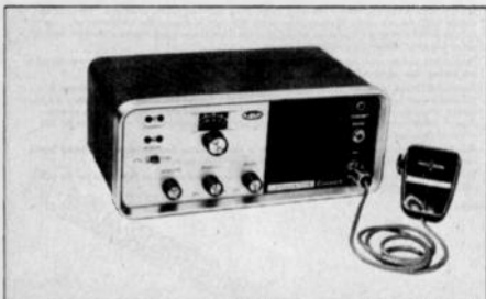
The Comsat 9 was a low cost rig which offered front panel crystal sockets which could be used for instant supplementation of the rig's internally installed crystals. Most folks used the external sockets for out-of-band operations, I'm afraid.
